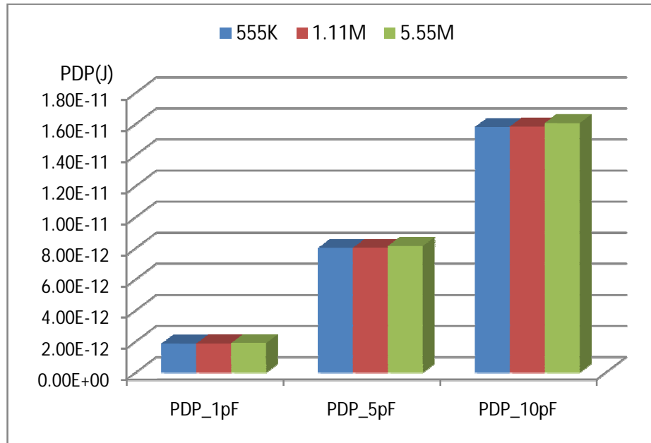
Figure 5.5: PDP product of TNOR for different capacitive load and frequencies
